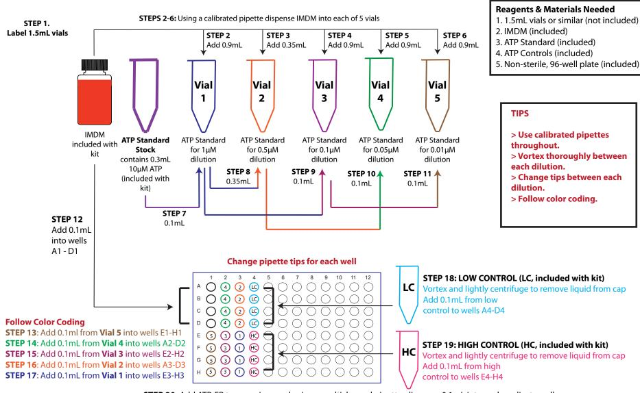
STEP 20: Add ATP-ER to reserviour and using a multichannel pipette, dispense 0.1mL into each replicate well
